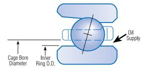
Fig. 17. Lubrication window for B-type bearings.
