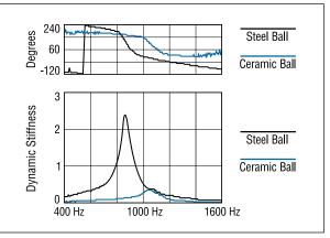
Dynamic stiffness analysis shows better rigidity and higher natural frequency for hybrid bearings.
