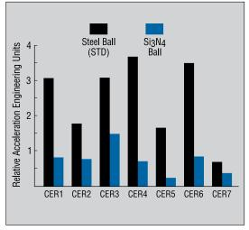
Vibration tests comparing spindles with steel ball bearings and the same spindle retrofit with ceramic hybrids. Vibration levels averaged two to seven times lower with silicon nitride balls.
