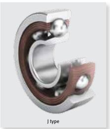
Non-Separable Type (J): Outer ring has full shoulders, inner ring has one shoulder cut away with a small retaining lip at the edge of the raceway.
