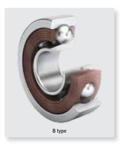
**Separable Type (B):** Outer ring has full shoulders, inner ring has one shoulder cut away. The inner ring is removable for mounting on the shaft separately from the outer ring assembly.
