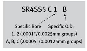
Fig. 24. This drawing, grossly exaggerated for clarity, illustrates specific calibration options (inch) for bore and O.D.
