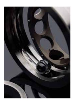
Barden super precision bearings come in inch or metric dimensions with diameters ranging from 4mm (5/32") OD up to 300mm (11½") OD. A variety of seals, shields and metallic/non-metallic cage designs are available to meet most requirements. Many Barden bearings operate comfortably at speeds reaching 2 million dN (bore in mm x RPM), or above.
